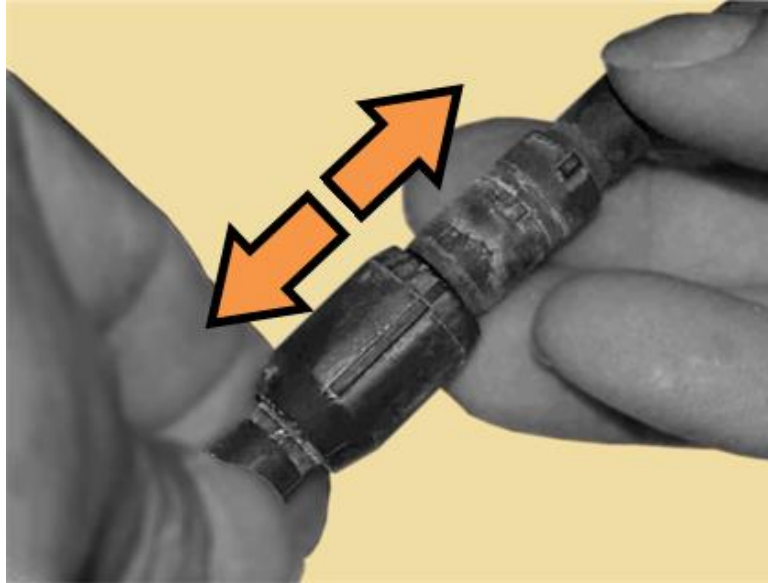
Figure C-15. Disconnect the Fan Power Supplies
